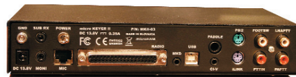
The rear panel is fairly uncluttered. Transceiver-specific interface cables plug into the large D socket.
